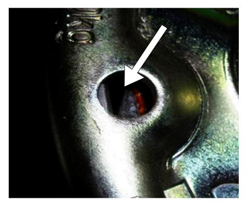
Through the outside hole you can inspect the condition of the brake lining. If the lining is worn to the end of the chamfer, it has to be changed because it is **not possible any more** to adjust the brakes.
