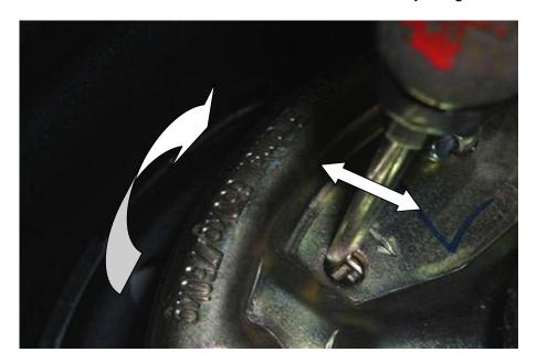
See on this picture how to move the starwheel arrowwise with a screwdriver. While adjusting, turn the wheel slowly in driving direction. Continue until the wheel blocks. Then move the starwheel back against the arrow (still turning the wheel in driving direction) until you can hear and feel that the brake lining is very, very smoothly touching the brake drum. If the lining is worn unequal, you may have to do this again several times.
