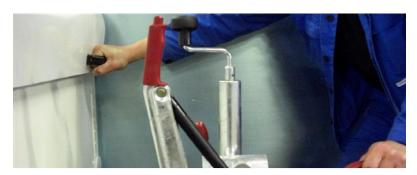
**Test:** Activate the hand brake and push the trailer back by hand .
