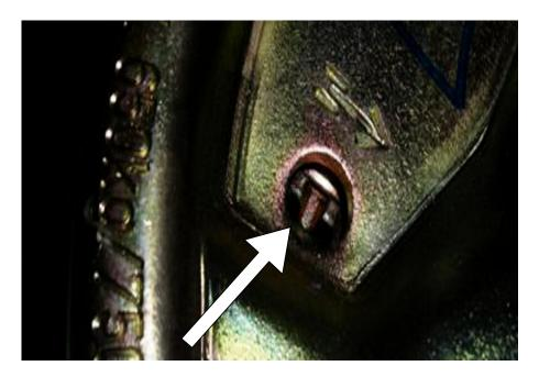
Through the second, inner hole you can see the starwheel for adjusting the brakes. The impressed arrow on the side of the hole shows the direction for adjusting.
